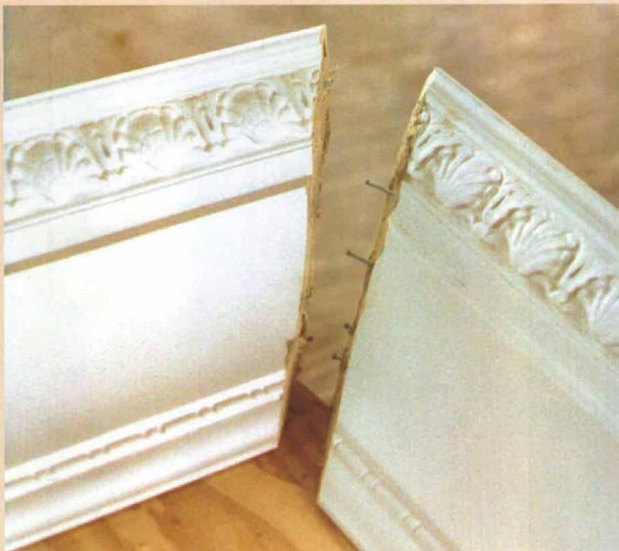
**Don't think you can save money by using the cheap stuff.** As a test, the author glued up one joint using the manufacturer's adhesive and another one with standard construction adhesive. The joint made with standard adhesive (photo above) was easily pulled apart, but the one made with the manufacturer's adhesive was stronger than the molding itself (photo below).
