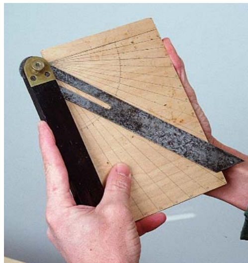
A homemade bevel board reveals the angle of the miter.
