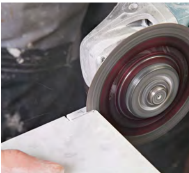
Notch the shelf. Use the same method for notching the sides to notch the shelf's leading edges.
