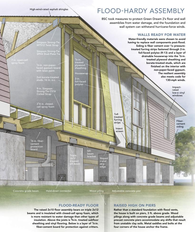
cell spray foam, if there's a problem, you have to scrape it away and then either get a Froth-Pak [to patch it] or hire someone to restore it," Reichel says. "But it's an easier first install, and you can do it no matter how high off the ground you are. Plus, it's a bit less expensive than the rigid-foam-board system, when you factor in the installation cost."
