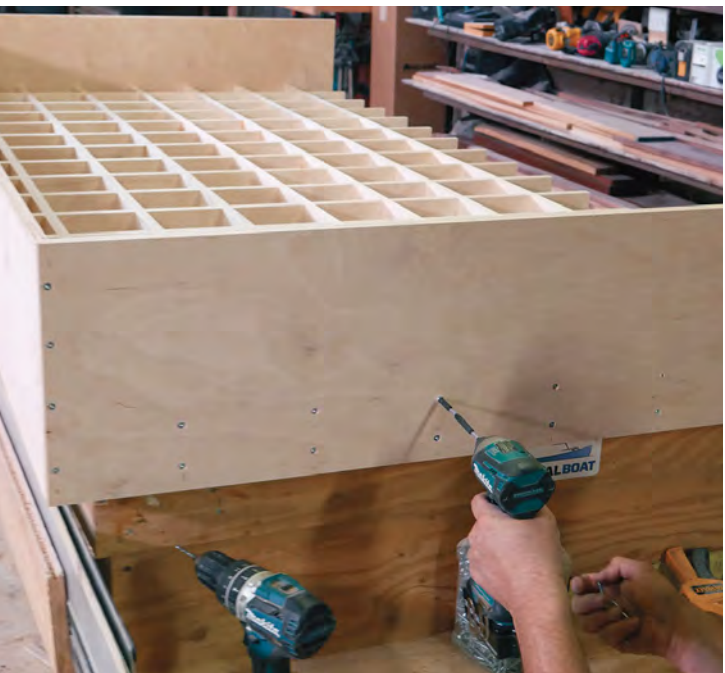
Add the apron. Tack the pieces of 12-in.-tall apron in place first, then fasten them with two countersunk 2-in. wood screws into the ends of each grid strip and four into each corner, keeping the screws at least 1 in. down from the top to protect sawblades when the table is in use.
