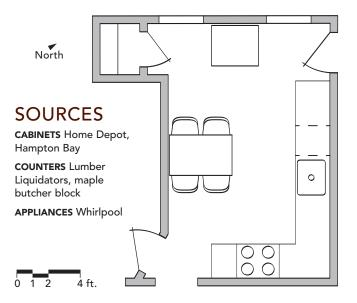
Although appliances were moved to accommodate the new dishwasher, the kitchen's original footprint and window and door layout stayed the same. This simplified construction by eliminating structural modifications and exterior work that's necessary when you move walls or change openings.
