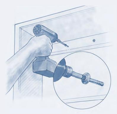
16-ga. nails, ensuring that I adequately nail my casing into my jamb. This locks the assembly together and secures it as one unit.
