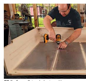
Fill the frame. Cut each sheet roughly 1½ in. larger than the openings in both directions, and predrill the sheets for the #6 washer-head screws so that the sheets don't distort when the screws are driven.
