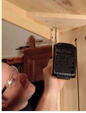
**Attach the top.** Drill pocket holes near the back of each side of the case, and drill elongated holes into the triangle corner blocks. The screws at the rear hold the top fast in place, while the screws in the elongated holes allow the top to expand and contract and minimize the risk of warping or cracking. If expansion does occur, it can only move outward, preventing a gap from opening at the wall.
