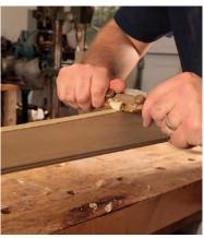
**Dividers need some handwork.** With the frame temporarily assembled with clamps, you can lay out the 2-in. divider locations on the rails and mark the mitered cuts and flat bottom of the joint using a combination square. The double-mitered ends of the dividers are easily cut with a miter saw set at 45°. For the rails, you can use a router and jig, a coping saw, or a
