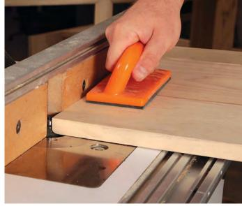
**Shape the top.** Using the router table, profile the ends first (across the grain) and then the length in order to minimize the chances of the corners blowing out deeper than the bit will cut.
