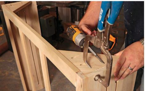
**Block it square.** Once the glue is set, replace the 90° clamping jigs with a pair of right-triangle blocks glued and pocket-screwed into the upper corners. Cut the blocks so that the grain runs parallel to the triangle's hypotenuse in order to maximize the strength of the joint. These triangle blocks hold the case square and provide a means of attaching the top.
