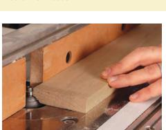
**Joint, rip, and profile.** For straight material and tight joints, run the stock through a jointer. Rip the rails to 3 in. and the stiles to  $2^{1}/4$  in. Profile one edge of each piece on the router table with a beading or cove bit.
